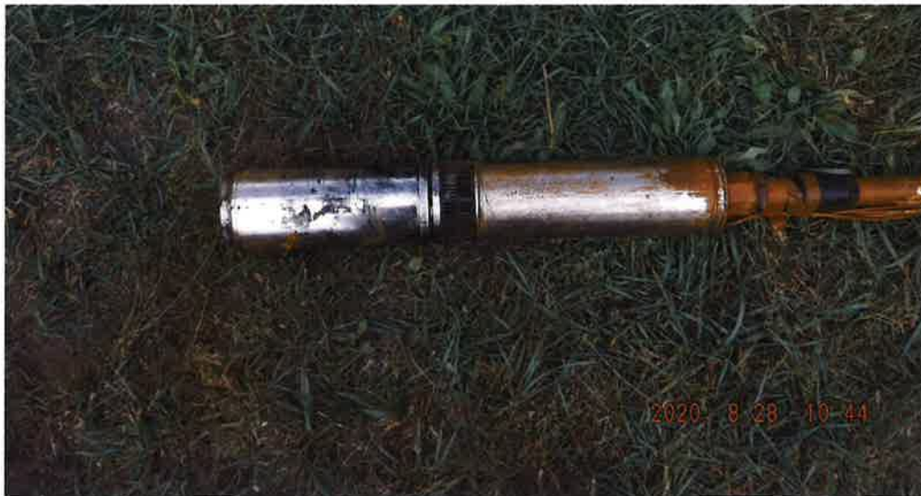
Figure B-2. Photograph of well pump and iron stained drop pipe
